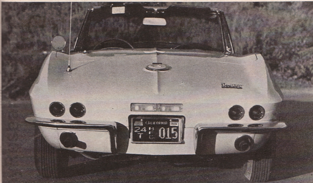
Standard, horizontal back-up light throws excellent beam, distinguishes '67 Sting Ray.
