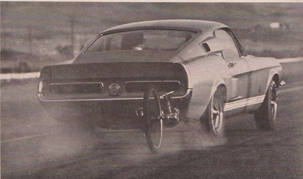
"Speedway 350" tires break loose easily, but need to for the best acceleration times.
