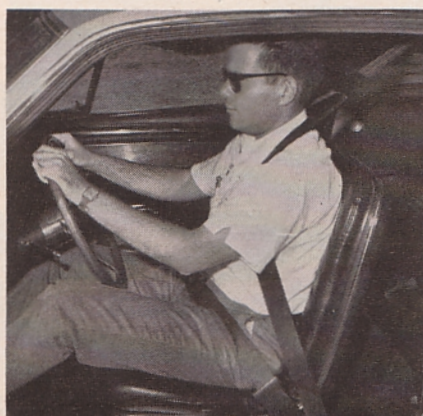
Inertia retractors stop sudden motion of GT wearer; allow slow, easy movement.
