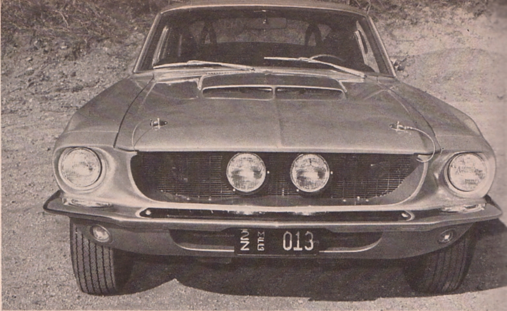
Nose and hood of GT are fiberglass items. Scoops deposit air on top of carburetors.
